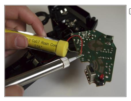
Replace the motherboard. Solder the wires back on to the new motherboard using the soldering kit. The black wire should be on the left and the red wire should be on the right.
