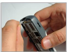
• With the motherboard and LCD unit removed, gently pull the power button out of its housing.
