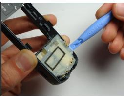
Pry out the power unit once the metallic plate has been removed.
