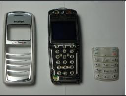
With the faceplate removed, simply peel off rubber key pad and remove.
