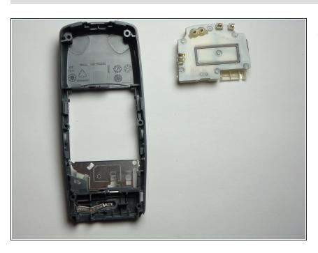
Be sure to place the power unit back into the phone's case with the gold hardware pointing upward.
