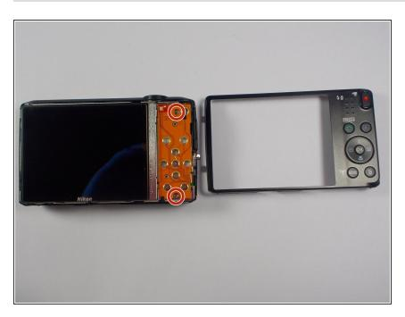
Using the Philips #00 Screwdriver, remove the two screws that are holding the keypad.
