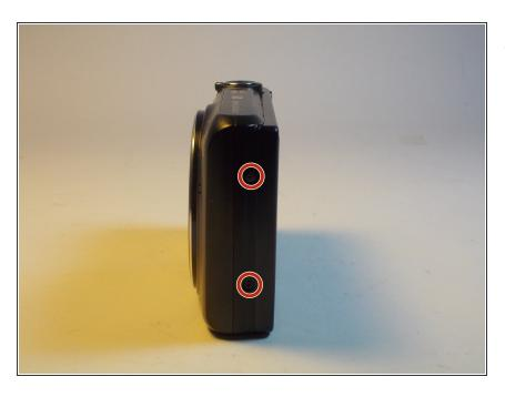
Rotate the camera to the left side and remove the two, black, #00 Philips screws.
