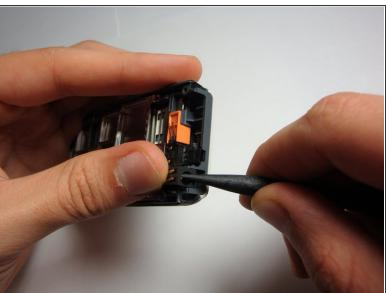
With the logic board and LCD unit removed, gently pry out the charging port.
