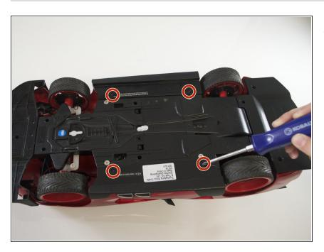
Remove the four 3 mm screws from the bottom panel using a 3 mm
