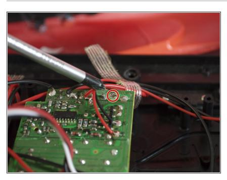
Replace motherboard. Place the new motherboard in the same position of old motherboard and replace the 3mm Phillips #2 screws.
