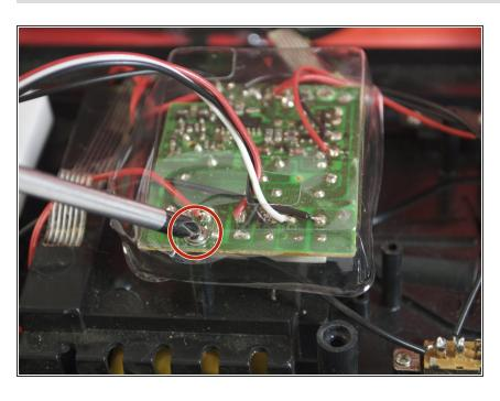
Unscrew water shield. Remove the 6mm Phillips #2 screw that is holding the water shield in place.
