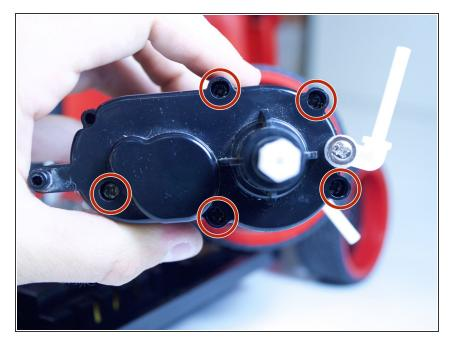
Remove the five 6mm Phillips #2 head screws from the left side of the motor housing.
