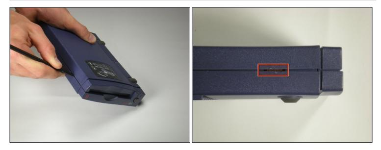
• Push in the plastic tab that can be seen through cracks in the front left corner using a spudger.
