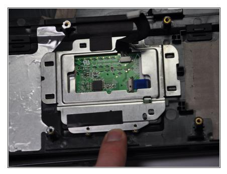
Slowly slide the frame in the direction of the keyboard hole on the plastic panel until the frame is released from the metal latches.
