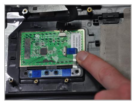
Carefully slide blue plastic connector on the mousepad towards the screw holes.
