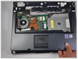
Using the iFixit opening tool, pry the black plastic panel (with mousepad) off of the motherboard.
