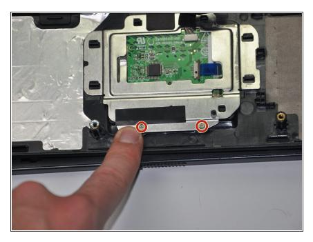
Remove the two 3.5mm Phillips #00 screws located at the bottom of the aluminum frame.
