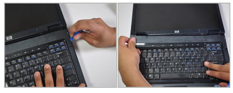
Using the iFixit opening tool, remove the plastic panel located between the keyboard and monitor.
