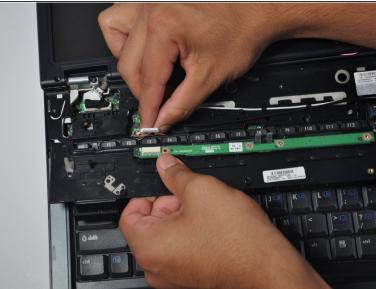
Remove the white cable attached to the just-removed plastic panel from the motherboard.
