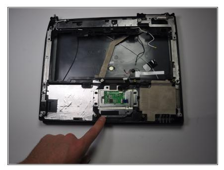
Find the green chip encased by an aluminum frame on the underside of the plastic panel that was removed last in the computer disassembly guide.
