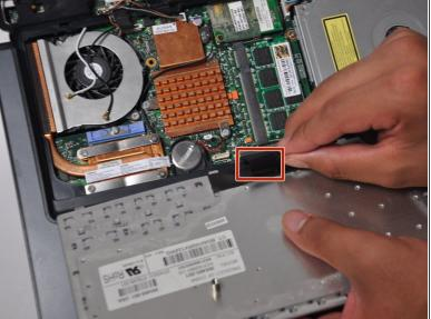
Flip the keyboard away from the monitor, rotating it so that the keys are face down on the mousepad. Remove the black cord at the bottom of the keyboard that connects it to the motherboard. The keyboard is now free and can be removed.
