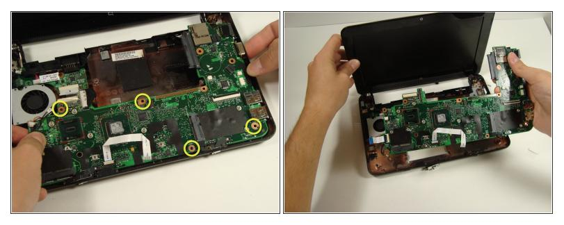
• Unscrew the 4 screws and lift the board out.
