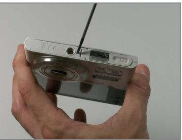
• Remove the four Phillips 2.381 mm screws on back side of camera and one Phillips 2.381 mm screw on the bottom of the camera, using a Phillips #00 screwdriver.
