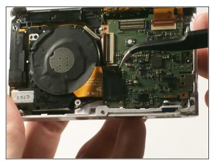
Use the <u>tweezers</u> to remove the black electrical tape covering the copper connector to the control board.
