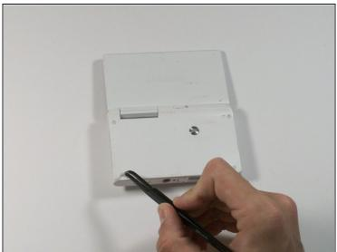
• Use <u>tweezers</u> to remove the four rubber screw covers.
