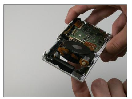
From the front of the camera, push the lens through the back of the camer.a
