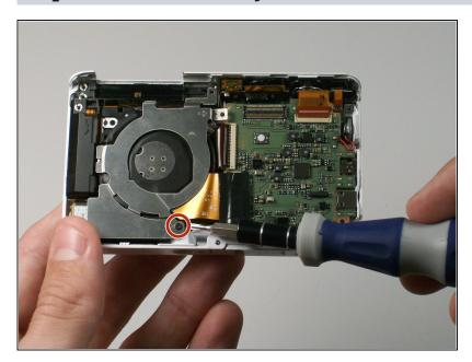
Remove the 2.381 mm screw with a Phillips #00 screwdriver.
