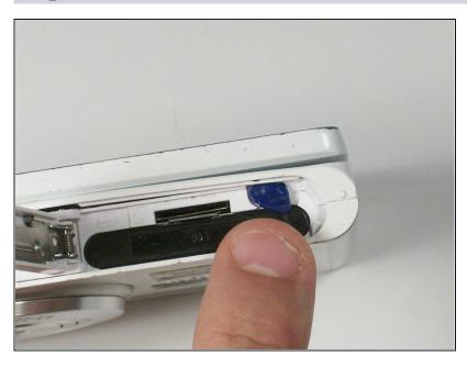
Push the blue battery holder up in the direction of the arrow.
