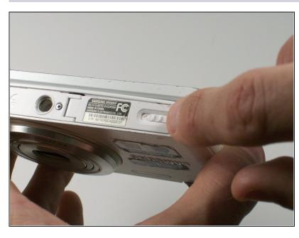
Slide the lock towards the middle of the camera, in the same direction of the arrow.
