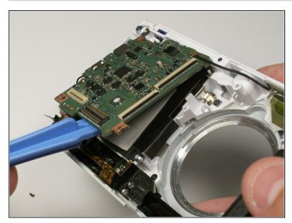
Use the plastic opening tool to pry the control board up, thus allowing the flash bulb assembly to be removed.
