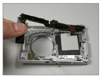
Beginning with the battery on the side, gently pull upwards to remove the entire flash bulb assembly.
