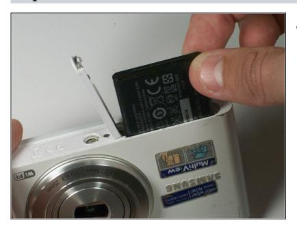
Pull the battery out of the battery slot.
