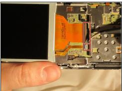
• Using the tweezers, lift the hinges connecting the two ribbon wires to the camera.
