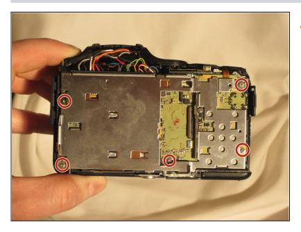
Remove these five Phillips screws, from the back of the camera, with the Phillips screwdriver.
