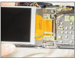
Remove the front casing to expose the LCD screen and wires.
