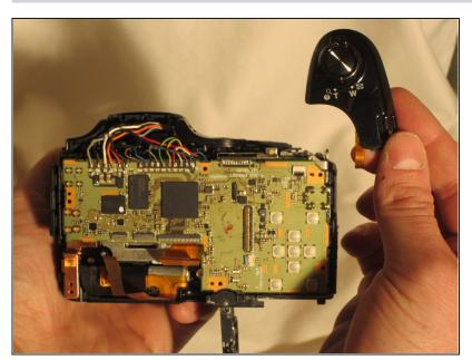
Remove the panel containing the shutter and zoom slider, by lifting it up.
