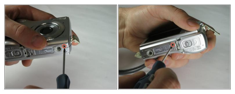
Remove the 2 exposed screws on the bottom of the camera.
