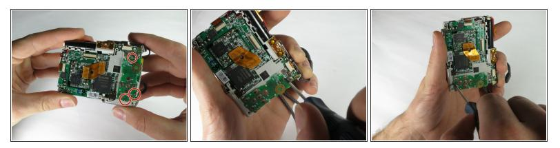
Remove the three screws holding the outer circuit board in place.
