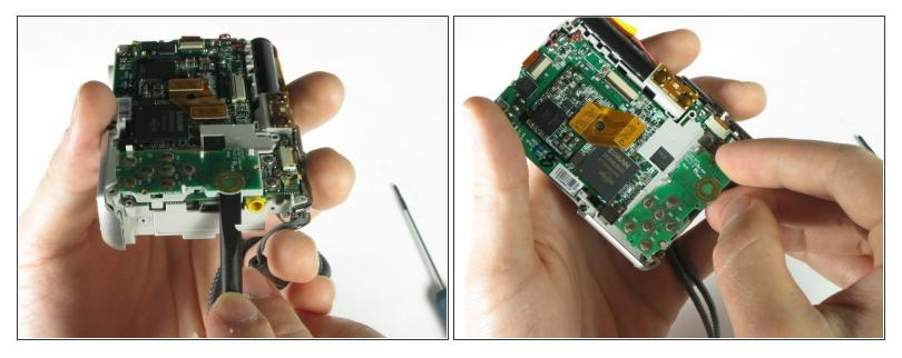
• Use the spudger or your fingers to remove the outer circuit board from the camera.
