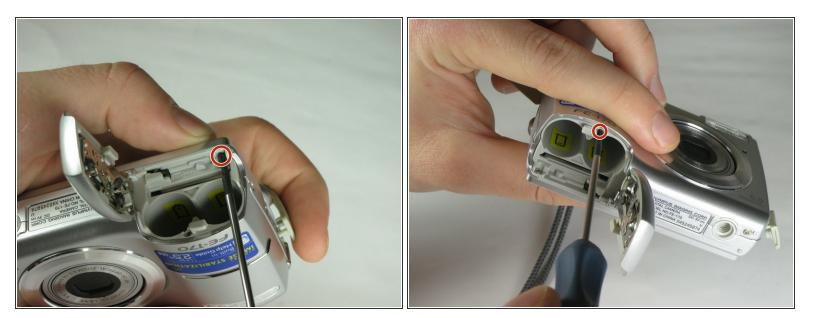
• Open the battery compartment and remove the 2 screws in the top of the opening.
