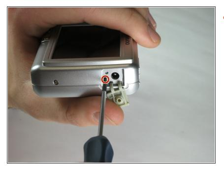
Uncover the video cable port on the side of the camera and remove the screw
