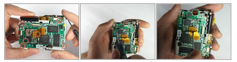
• Remove the screws shown using the 00 philips screwdriver.
