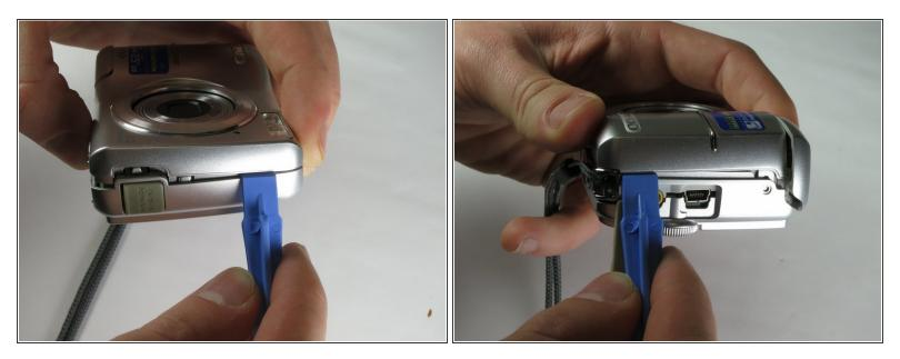
• Loosen the panels on the sides of the camera in the shown places by slipping the plastic opening tool in the crack between the panels. Lightly apply pressure.
