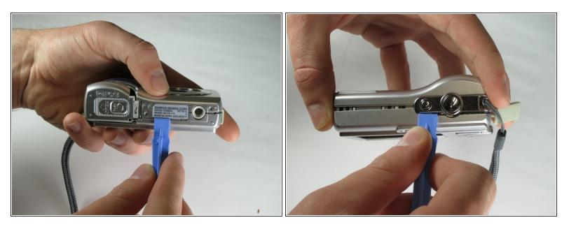
• Carefully slip the head of the plastic opening tool under the panels by finding the crack between the panels. Lightly apply pressure in the shown places at the top and bottom of the camera.
