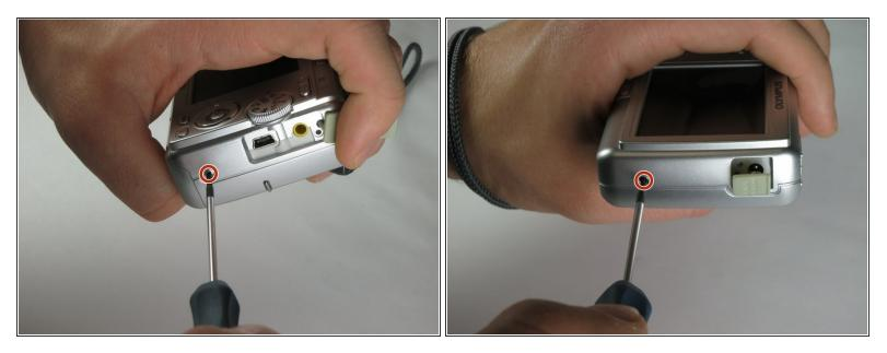
Remove the 2 exposed screws on opposite sides of the camera. Turn the screws counterclockwise to remove.
