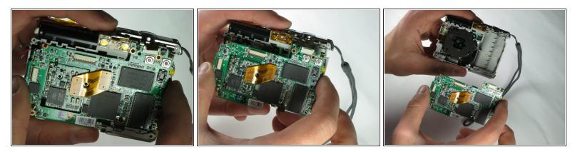
• Gently pull the motherboard (from the bottom first) away from the device.
