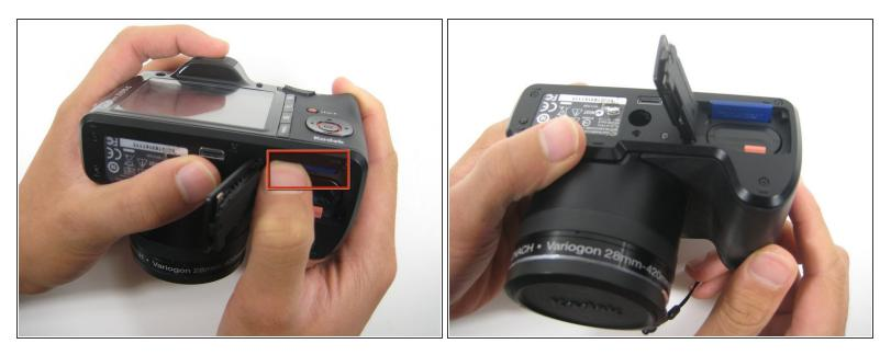
• After locating the SD card, gently push down on the card and release. This will cause the SD card to pop out of its position in the camera as shown in the second picture of this step.
