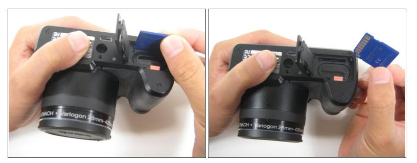
After removing the SD card from its locked position, gently pull the SD card out from the container to successfully remove it from the camera.
