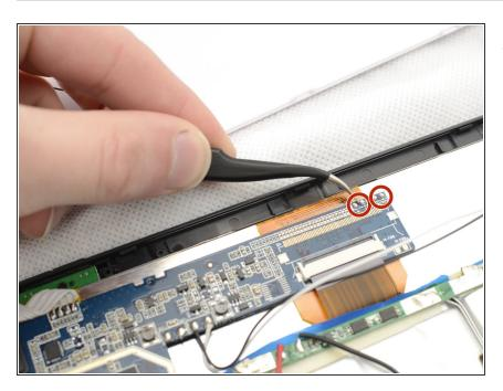
Check to see if the wires of the speakers are connected to the motherboard assembly here.
