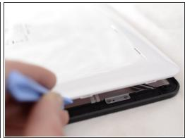
• Pry along the edge of the device to separate the back cover from the device.
