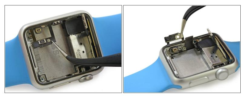
• Given the limited amount of <u>space</u> inside the Apple Watch, we find the microphone ribbon cable creatively ensnared between the inner and outer layers of the case.
