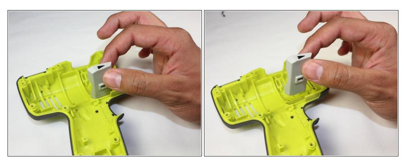
• Lift up on the direction toggle to remove it from the case.
