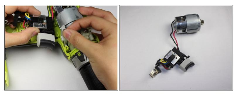
Holding the direction select switch in place, grip both sides of the trigger assembly and lift it up and towards the base of the drill.
