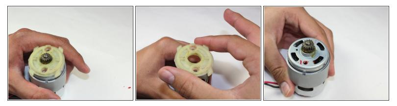
• Remove the plastic spacer by lifting it straight up.
