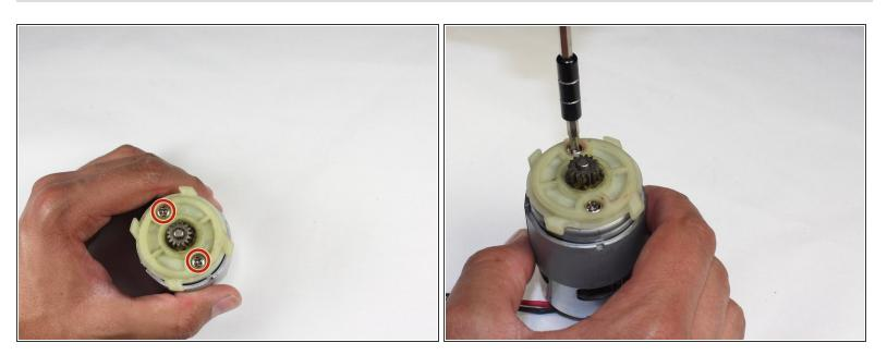
Unscrew the two 10mm Philips #1 screws to remove the plastic spacer. Be careful not to lose the metal ring washers that come with the screws.
