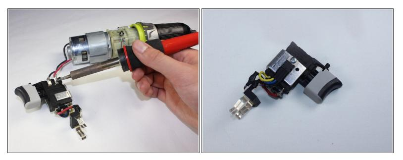
• To separate the trigger assembly from the motor, use a soldering iron to melt the solder and pull gently on the red and black wires from the trigger.
