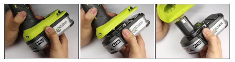
The battery can shock you. Only touch plastic, non-conductive components.
