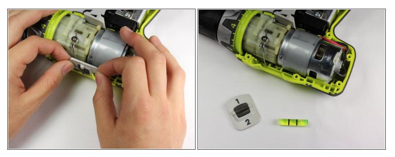
• Lift the gear switch upwards from the top of the drill head.
