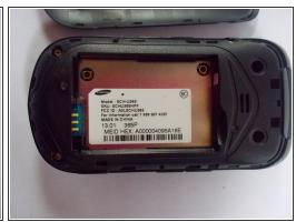
Pop out the battery by placing your finger in between the open slit.
