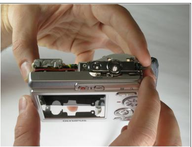
Ensure that the panels have been loosened. Carefully use hands to pull back and remove the panels. To reassemble your device, follow these instructions in reverse order.
