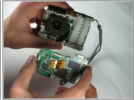
Gently pull the motherboard (from the bottom first) away from the device.
