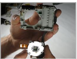
Gently remove the lens assembly by pulling on the top of the assembly first, then removing from the device.
