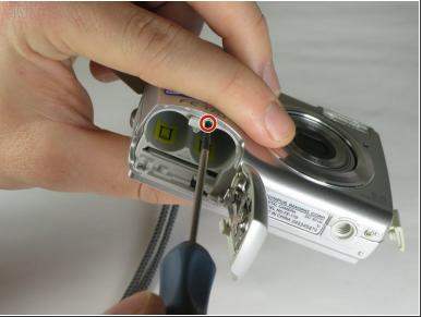
Open the battery compartment and remove the 2 screws in the top of the opening.
