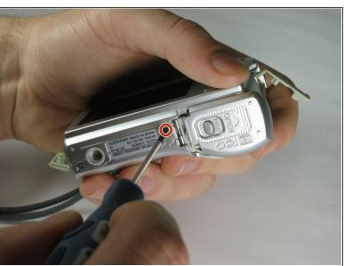
Remove the 2 exposed screws on the bottom of the camera.
