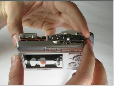
Ensure that the panels have been loosened. Carefully use hands to pull back and remove the panels.
