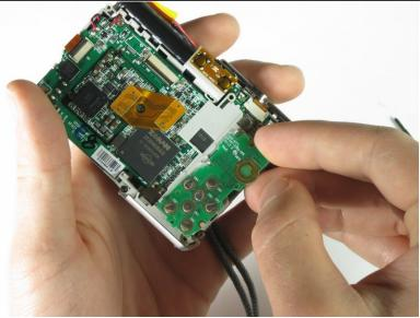
Use the spudger or your fingers to remove the outer circuit board from the camera.
