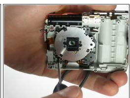
Remove the 3 screws holding the lens assembly in place.
