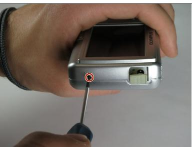
Remove the 2 exposed screws on opposite sides of the camera. Turn the screws counterclockwise to remove.
