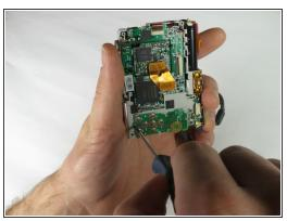
• Remove the three screws holding the outer circuit board in place.
