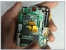
• Remove the screws shown using the 00 philips screwdriver.
