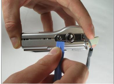
• Carefully slip the head of the plastic opening tool under the panels by finding the crack between the panels. Lightly apply pressure in the shown places at the top and bottom of the camera.
