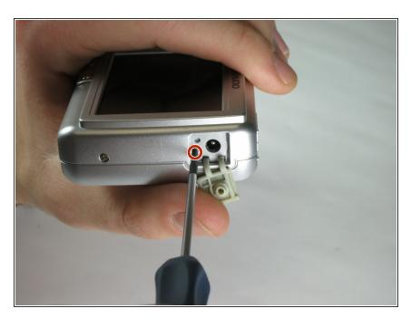
Uncover the video cable port on the side of the camera and remove the screw
