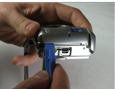
Loosen the panels on the sides of the camera in the shown places by slipping the plastic opening tool in the crack between the panels. Lightly apply pressure.
