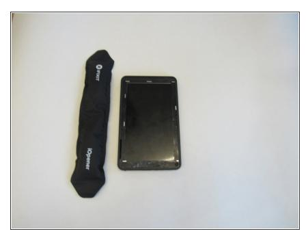
Heat the iOpener in the microwave, following the instructions provided with the tool. Lay the heated iOpener on the front screen for two minutes to soften the connection of the screen to the tablet.
