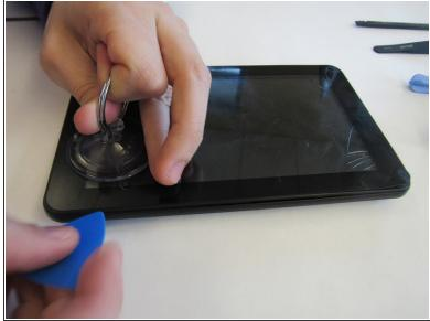
Use the suction cup and plastic opening tool to pry the front screen from the tablet.
