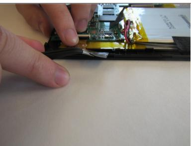
Using the tweezers, remove the black tape connecting the screen to the motherboard.
