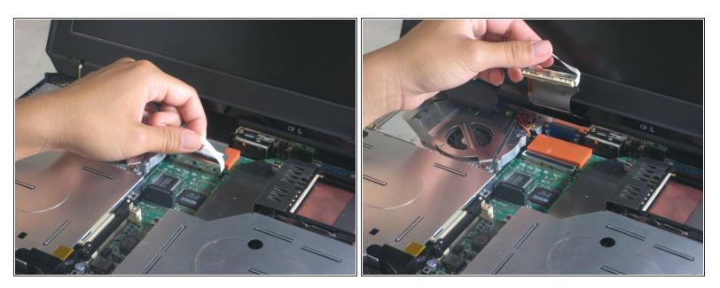
• Pull out the white tab connecting the LCD to the motherboard.
