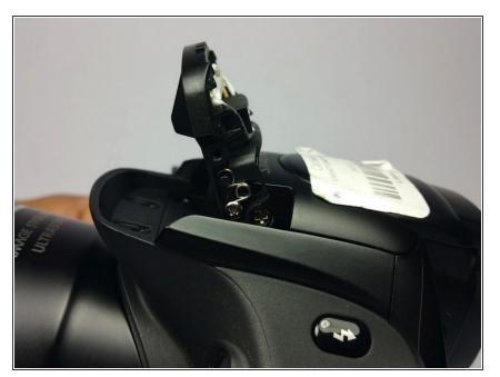
Replace the external flash cover or the internal flashlight when all 6 mm silver screws are out.
