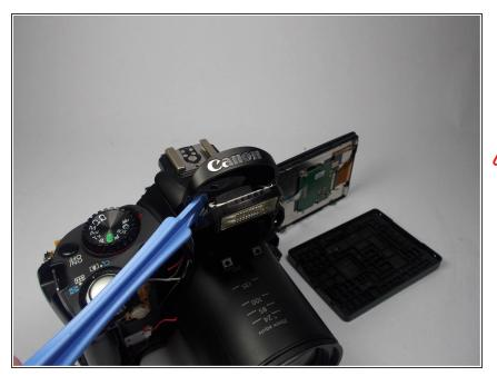
Remove the plastic cover using the iFixIt Plastic Opening Tool.
