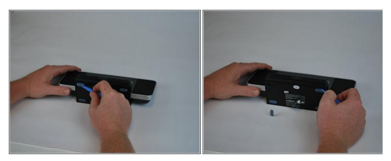
• Using a plastic opening tool, peel off the adhesive gel stoppers.
