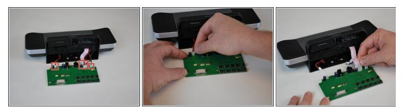
• Disconnect the four cables connecting the motherboard to the device.
