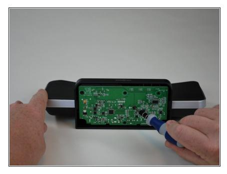
• Use a Phillips screwdriver to remove the 9.5 mm screw located near the center of the motherboard.
