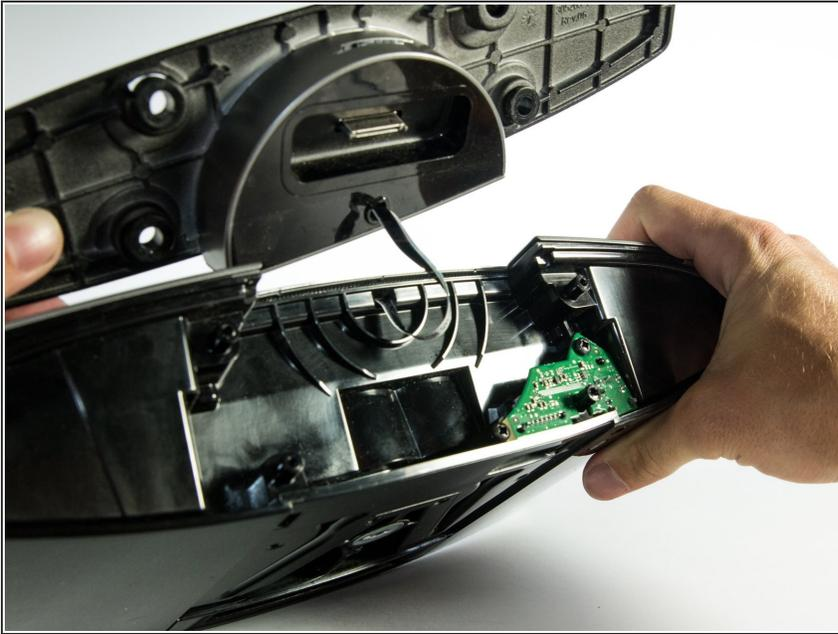
**⚠** Once the panel is removed you will see a ribbon connecting the dock to the speaker. Be careful to orient the speaker so that you can work on the dock connector without pulling on the ribbon!
