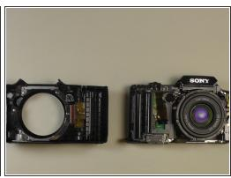
Pry the front cover of the camera off with the plastic opening tool.
