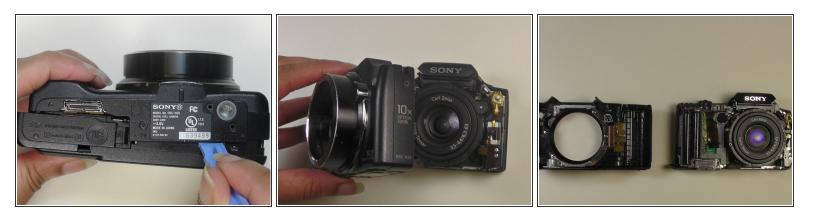
• Pry the front cover of the camera off with the plastic opening tool.
