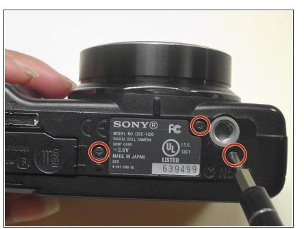
• Remove all three screws from the bottom of the camera.
