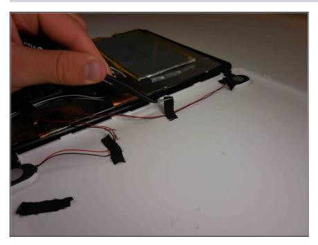
Remove the tapes one by one from the connecting wires with tweezers.
