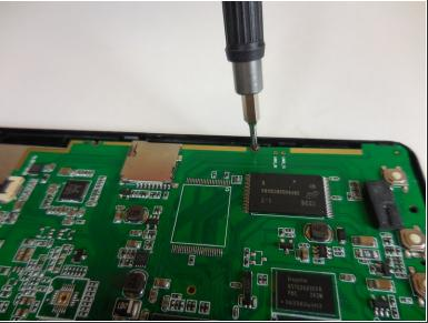
• Use a Phillips #000 screwdriver to remove the three screws from the motherboard.
