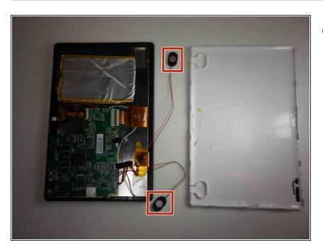
Pull the speakers away from the back casing carefully.
