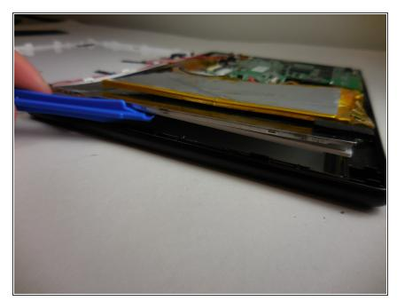
Use the plastic opening tool to pull the metal and plastic plates away from the interior of the tablet. Slowly pop each tab off until the plates are mostly separated from the base.
