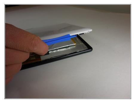
Remove the back casing by slowly popping each tab out with a plastic opening tool.
