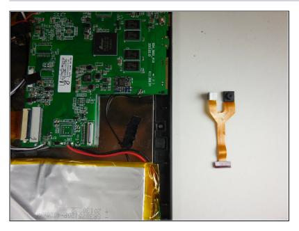
Pull the copper connection carefully away from the motherboard of the tablet to completely remove the camera.
