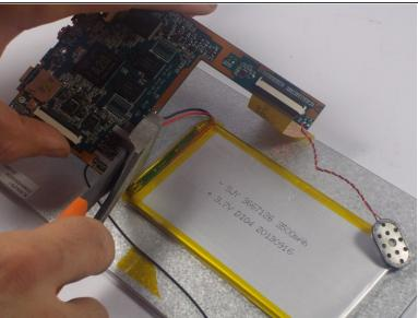
The two wires connecting the battery are located within the yellow box. They are soldered to the motherboard and must be cut. Using a pair of wire cutters cut each wire as close to the board as you can without damaging the board.
