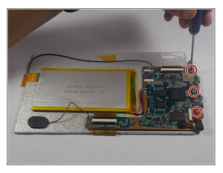
Before removing the battery it is necessary to detach the motherboard to allow yourself more room and to prevent damage. To do this remove the three Philips head screws marked by the red circles. These screws are also 1cm in diameter.
