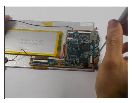
With the new battery connected you can now re-secure the motherboard with the three screws you previously removed.
