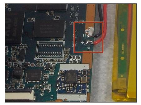
Before connecting the new battery to the motherboard locate the positive and negative wire locations.
