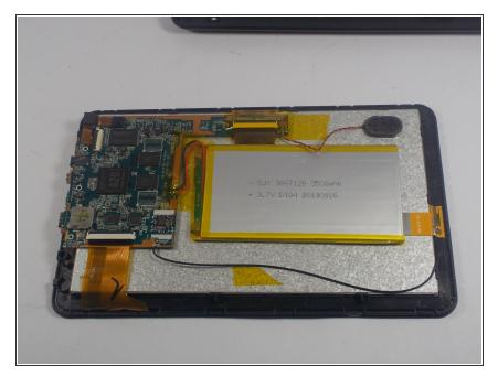
First locate the battery on the tablet, all of the battery information is printed on the top of the battery.
