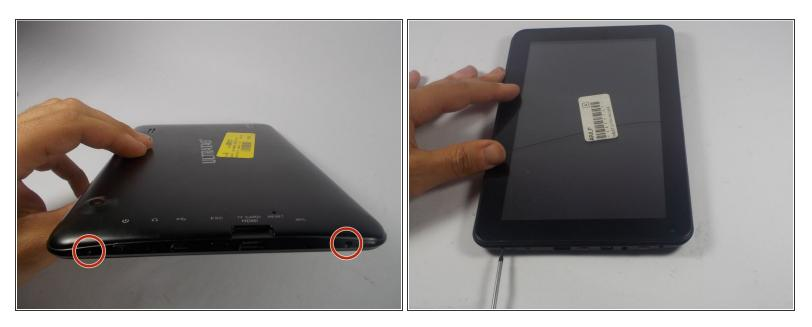
On the top of the tablet there are two 1cm screws that hold the back cover on. Locate these screws and remove them using a Phillips head #0 screw driver.
