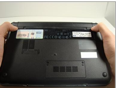
Locate the battery and the battery tabs on the bottom of the Compaq Mini.
