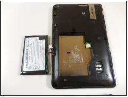
• Use the plastic spudger to lift the battery up and away from the device.
