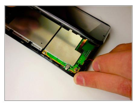
Locate the red and black wire connected to the logic board with the round, black, rubber disc that connects to the other half of the device. Gently pull the wire up from the logic board.
