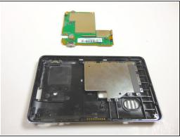
Starting near the power button, leverage the spudger to pry up the logic board around the perimeter of the frame.
