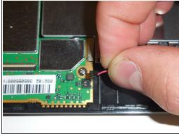
Separate the connection between the speaker and the logic board by gently pulling the wire up.
