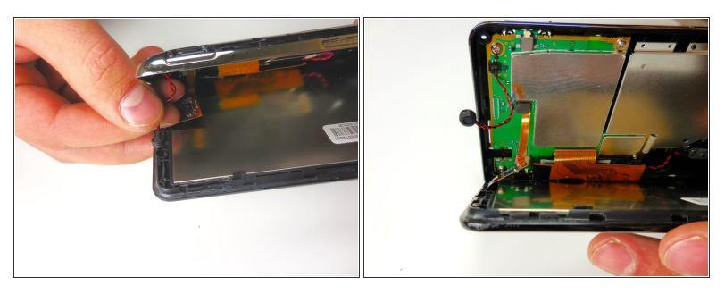
Using your fingers, remove the red and black wire from the back of the screen.
