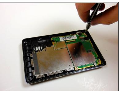
Using the J000 bit, unscrew the four 4.0 mm screws from the corners of the logic board.
