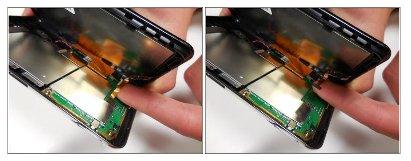
Pull up on the smaller orange tab with your finger from the circuit board.
