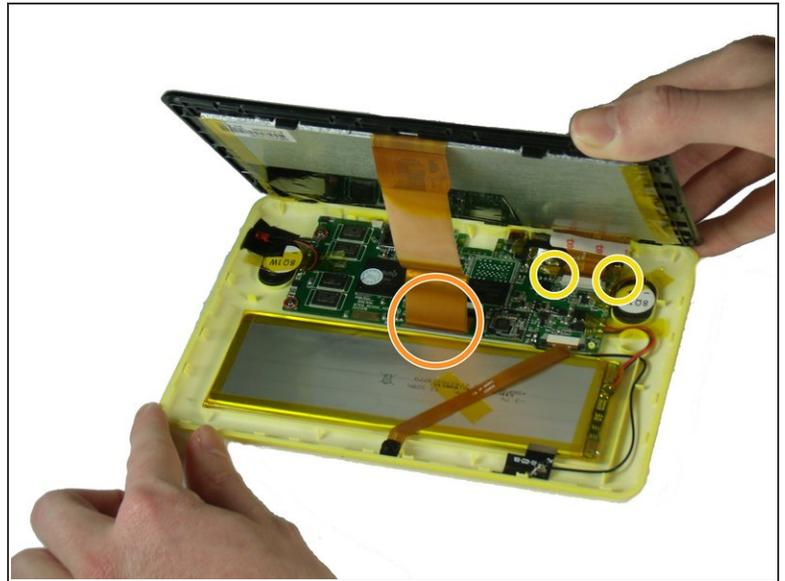
**!** Be careful not to damage any wires or ribbon cables during this step.
