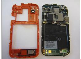
• Use an opening tool or a spudger to gently remove the rear frame.
