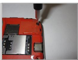
Use a Torx T5 screwdriver to unscrew and remove five 3.0 mm screws from the rear frame.
