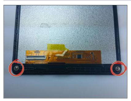
Remove the two silver screws from the bottom of the device.
