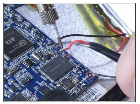
Apply heat to the solder holding each of the black and red wires to the circuit board while gently pulling with tweezers. When hot enough, the wire should pull away freely from the joint.
