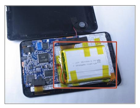
Locate battery and wires connected to the battery
