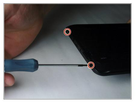
Unscrew the two 2.70 mm Phillips #00 screws on the side of the tablet that has the buttons and the headphone jack (bottom side when holding upright).
