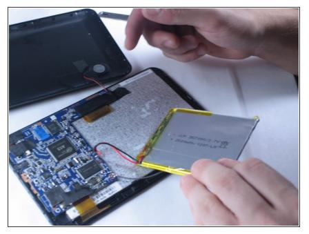
• The battery should now lift up freely from the device.
