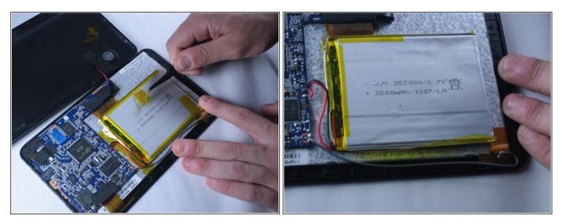
Using tweezers or your fingers, begin removing the yellow tape holding the battery down to the device.
