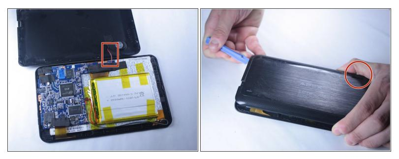
**CAUTION**: When removing the back panel of the tablet, take caution around the speaker. This is located in the lower right corner when looking at the back of the tablet. There are two wires inside connecting the tablet back panel to the device itself and this connection may be severed if the back is pulled off without care.
