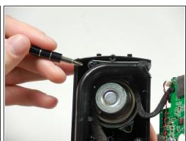
Remove screws that hold the plastic L-pipe in place.
