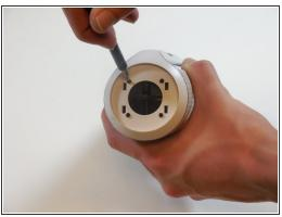
Unscrew four 3.3mm screws on each end of the JBL using a size 1 ph screw driver (8 screws total).
