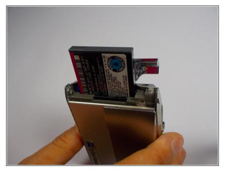
Remove battery and insert new battery according to the direction of the arrows on the battery pack.
