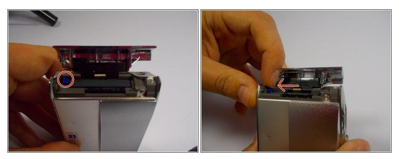
Push blue tab towards bottom of camera to release the battery pack.
