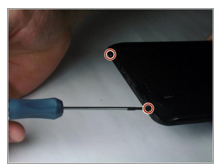
Unscrew the two 2.70 mm Phillips #00 screws on the side of the tablet that has the buttons and the headphone jack (bottom side when holding upright).
