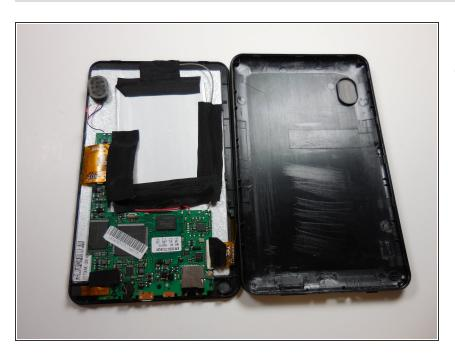
Once the speaker is disconnected, the cover removal is complete.
