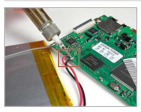
Remove the red and black battery wires from the circuit board with the solder removal tool.
