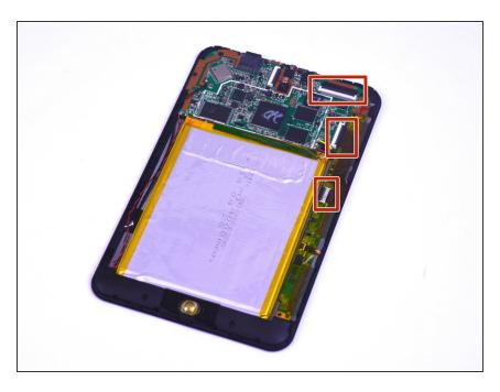
Unlock the three ribbon cable connector latches to remove the cables.
