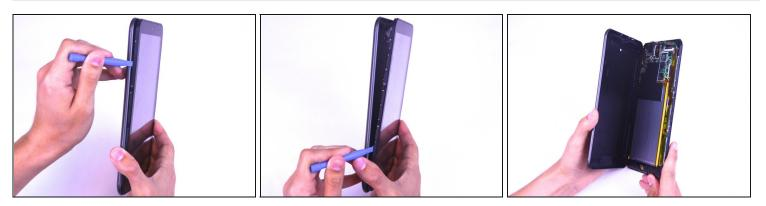
• Use an opening tool to pry open a corner of the device, then slide the tool down the side of the device to completely open it.
