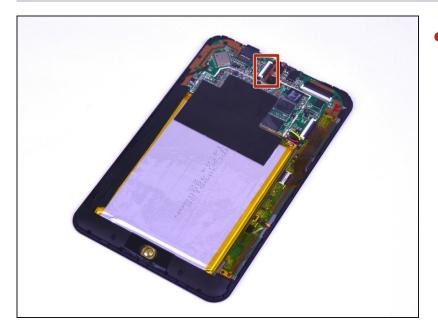
• Use your fingers to pull the latch upwards to unlock the ribbon cable.
