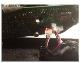
Remove the first two connectors on the underside of the motherboard.
