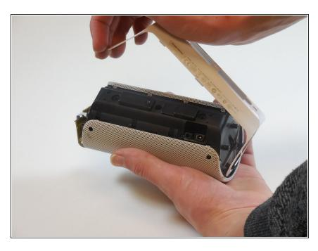
Remove last white back plate to expose the back of the speaker cover.
