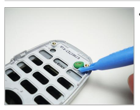
Use a plastic opening tool to lift the microphone out of its circular slot.
