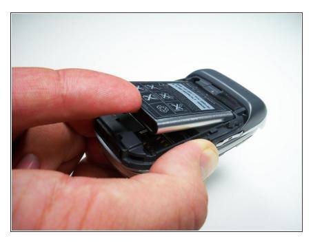
Using a fingernail lift the battery out of the phone.
