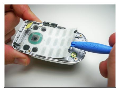
Using a plastic opening tool lift up the keypad to remove it.
