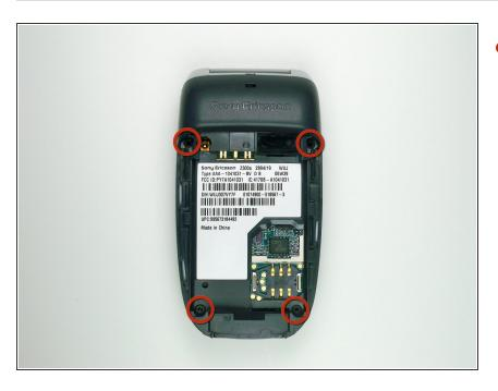
To remove the back case first remove the four screws shown with a T5 Torx screwdriver
