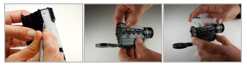
• Remove white piece by pressing a fingernail in notch (located in previous step) and lifting up on white piece.
