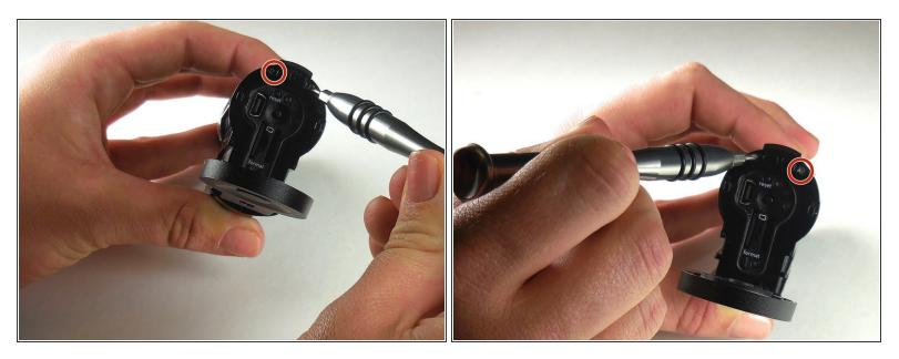
With the phillips head screwdriver (PH000) remove the two 3.31mm (.130inch) screws located at the top, **above** the reset button.
