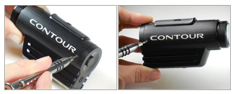
Using the phillips head screwdriver (PH000) remove the two 4.46mm (.175in) screws on each side near the back of the camera.
