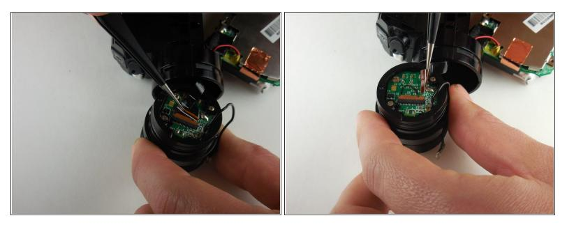
• Disconnect the ribbon connector connecting the lens unit to the logic board.
