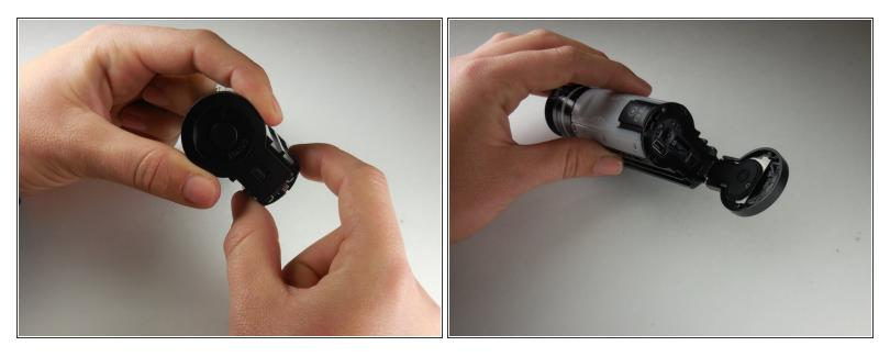
• Open the back door by your thumb and index finger on sides of back door and pull upward.
