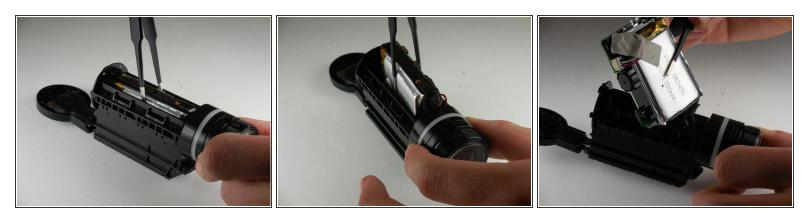
• Using flathead tweezers, remove the logic board and the battery from the camera.
