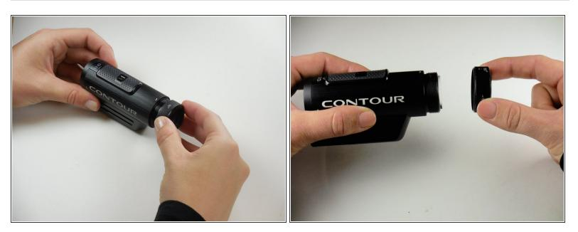
• Rotate the metal ring counterclockwise until completely removed.
