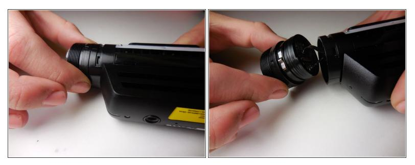
Twist lens unit until able to easily remove
