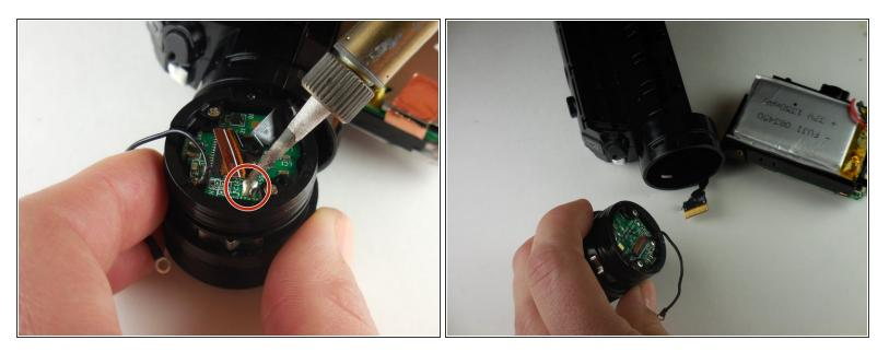
Remove the ribbon connecter from the lens unit by soldering.
