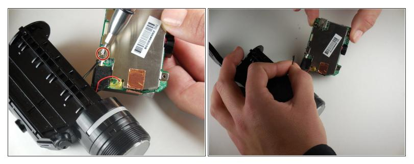
Using a phillips head screwdriver (PH 000), remove the screw connecting the lens unit to the logic board.
