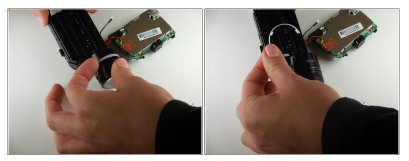
• Remove the semicircular white plastic strip near the lens unit.
