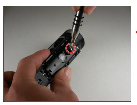
With a phillips head screwdriver (PH 000), remove the 5.54 mm (0.218 in) screw located next to the tripod screw-in.
