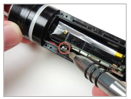
Using the phillips head size PH000 screwdriver remove 3.67mm (0.1445 inch) screw located on the side of logic board within the body of the camera.
