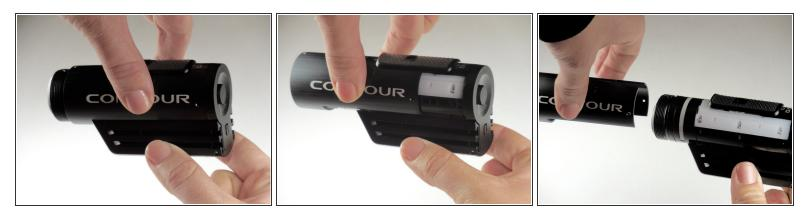
• Grab the camera on both sides and slide the outer shell forward until completely removed.
