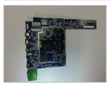
Gently lift the motherboard out of the tablet, make sure no wires are still caught or attached while you lift the motherboard.
