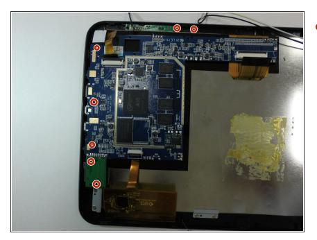
Remove the 3.5mm screws located at these locations shown on the picture by using the PH00 screwdriver.
