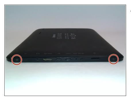
Remove the two 3mm screws using a PH00 screwdriver.
