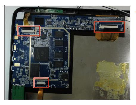
Remove contact strips by lifting gently on the clip indicated in this picture, then pulling strip out of the clip.
