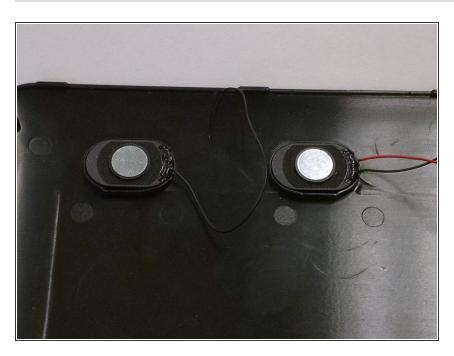
Glue the speakers flat against their respective sound output panels with the silver sides facing out/towards the interior of the tablet.
