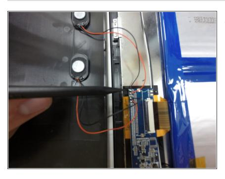
Solder the wires of the new speaker to the motherboard as shown in the image.
