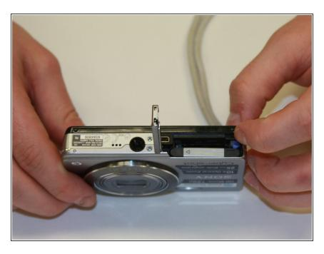
Open the battery lock to release the battery.
