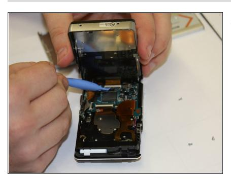
Carefully remove and replace the motherboard.
