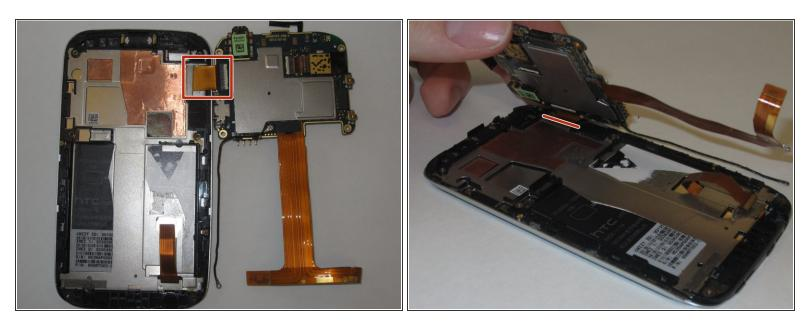
• Gently pry logic board from the casing by lifting the left side up, as if there was a hinge on the right, folding it over the right edge where you will see a gold/orange ribbon cable.
