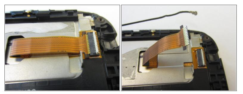
• Disconnect gold ribbon cable connecting screen to logic board by pulling cable out gently.
