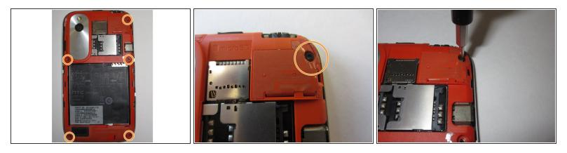
• Use a Torx T5 screwdriver to unscrew and remove five 3.0 mm screws from the rear frame.
