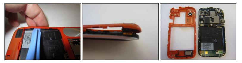
• Use an opening tool or a spudger to gently remove the rear frame.
