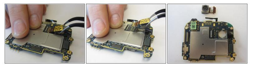
• Preferably using tweezers, gently pull the camera assembly up from the motherboard, and away from the connector and the ribbon cable will slide out easily.
