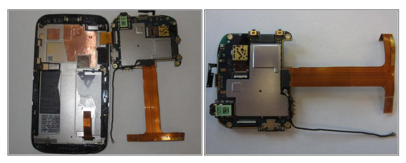
• Gently pull the logic board to the right and it will disconnect from the chassis.
