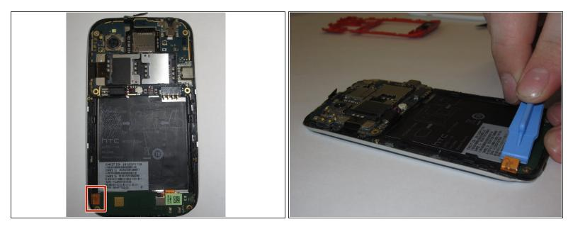
• Remove the connector on left side of the Navigation board by unplugging/prying the orange ribbon.
